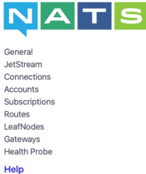
Figure 4.4: NATS UI. The UI can be used to perform server health-checks, or check live connections and subscriptions.
